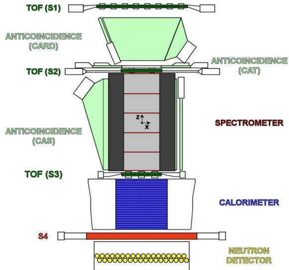
Fig. 1. the PAMELA experiment. From top to bottom, the first two TOF planes (S1 and S2) interleaved by the first module of the AC system (CARD), the magnetic spectrometer surrounded by the second AC device (CAS), the third TOF plane (S3), the imaging calorimeter, the bottom scintillator (S4) and the neutron detector. Total height is 1.3 m, weighting 470 kg. Average power consumption is 355 W.
