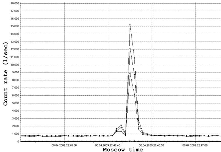
Fig. 5: Gamma ray burst on April 08, 2009. Count rates in three pairs of phoswich detectors
