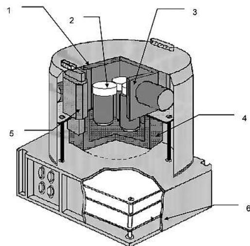
Fig. 1: The design of the "PENGUIN-M" detector block. 1: top shield detector (polystyrene+PMT); 2: detector-scatterer SD (paraterphenyl+PEM); 3: phoswich-detectors PD (NaI+polystyrene); 4: bottom shield detector (polystyrene); 5: soft x-ray detectors (proportional counters); 6: digital electronics plates
