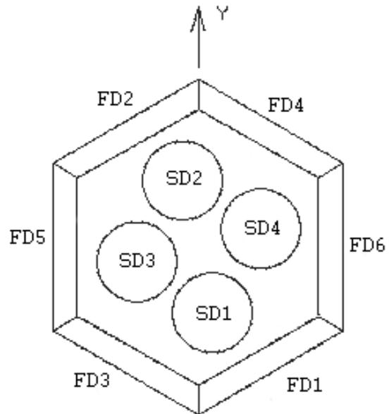
Fig. 2: The positioning of scatterer detectors (SD) and phoswich detectors (FD)
