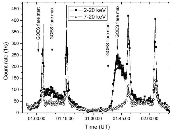
Fig. 4: Soft X-ray flare on March 26, 2009 as registered by soft X-ray detector detectors
