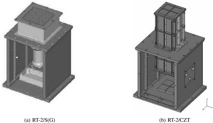
Fig. 1: Isometric view of RT-2/S (Phoswich detector) and RT-2/CZT (Solid-state detector). The different parts of the assembly (eg. collimator, HV box, PMT, CZT-CMOS mounting plate etc.) are seen in the drawing
