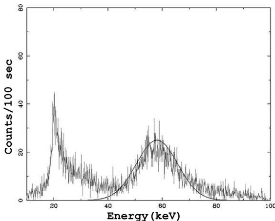
Fig. 9: A typical energy calibrated spectra of NaI(Tl) crystal (RT-2/G)
