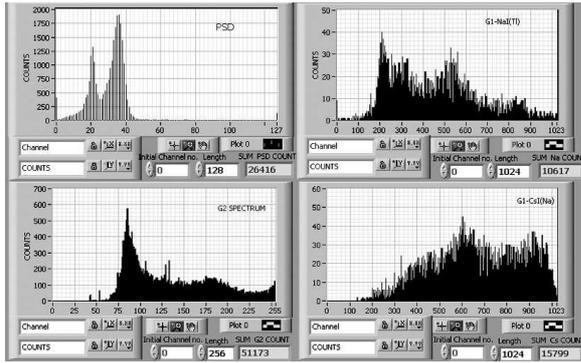
Fig. 7: Channel spectra (PSD, NaI(Tl), CsI(Na) and G2) of RT-2/S on April 16, 2009
