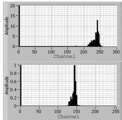
Fig. 11: The sample of CMOS calibration spectra observed in different parts of the orbit
