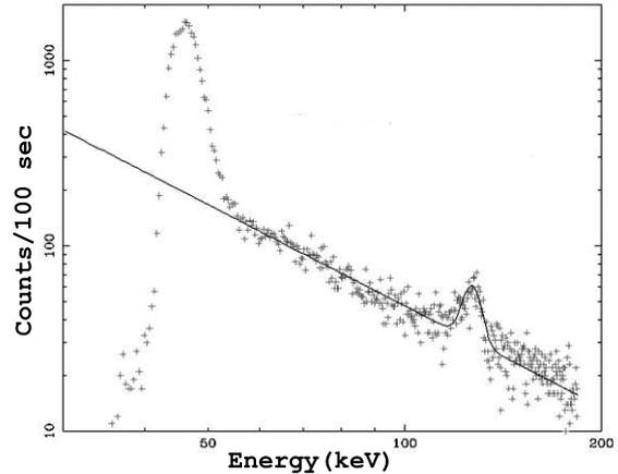
Fig. 10: Sample of CZT1 spectrum with calibration source peak of resolution 7.32% at 127 keV
