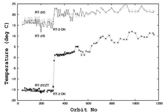
Fig. 2: RT-2 instruments temperature profile onboard "CORONAS-PHOTON" mission
