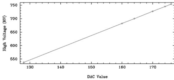
Fig. 4: Linearity calibration of HV operation of RT-2/S detector
