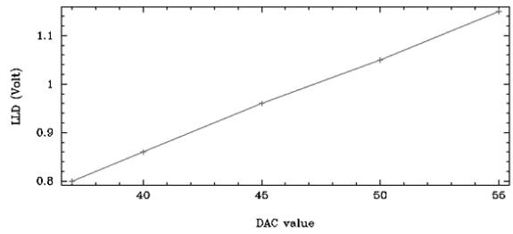
Fig. 5: Linearity calibration of LLD operation of RT-2/S detector
