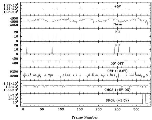
Fig. 6: Health parameters plot of RT-2/CZT on April 16, 2009
