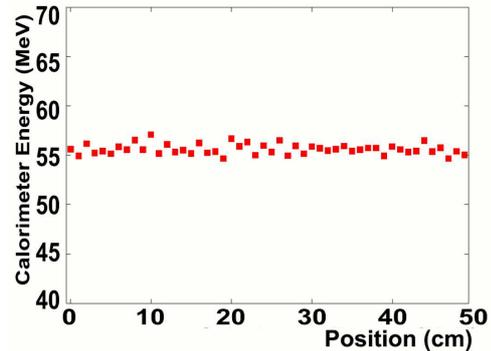
Fig. 7. Calorimeter energy with respect to the electron beam injection points.
