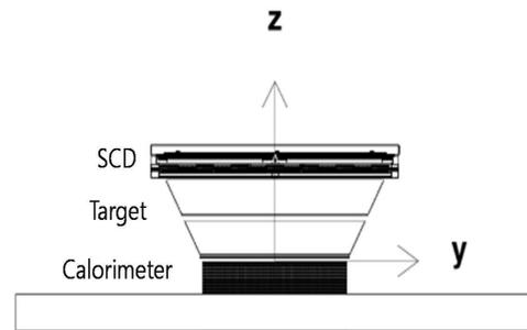
Fig. 1. Configuration of the CREAM calorimeter module.
