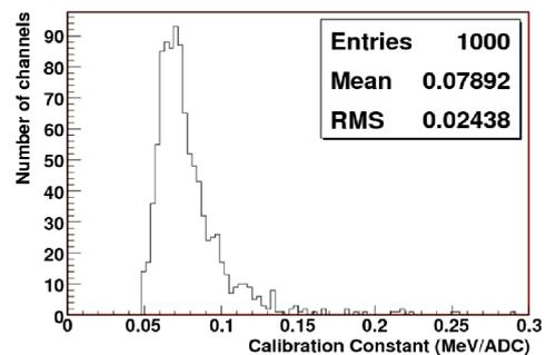
Fig. 3. A distribution of calibration constants for the CREAM-III calorimeter.
