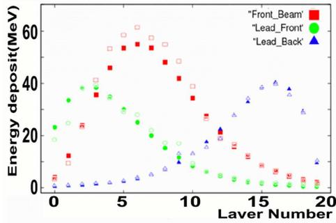
Fig. 4. Mean longitudinal profile of 150 GeV electrons – data (open symbols) and simulation (solid symbols).
