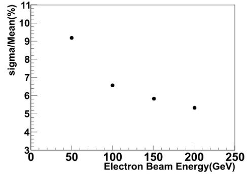
Fig. 6. Calibrated calorimeter resolution for different electron beam energies.
