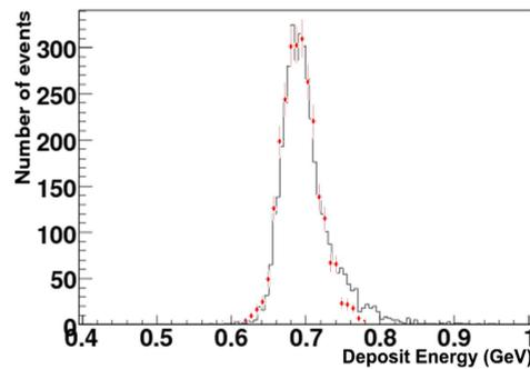
Fig. 5. Calorimeter energy distribution for 150 GeV electrons from simulations and beam data.
