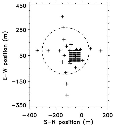
Fig. 1: Layout of the CODALEMA experiment showing the 24 dipoles (crosses), the 18 DAM elements (black rectangles) and the area (dashed circle) delimiting core footprints of the events reconstructed from surface detector array measurements.
