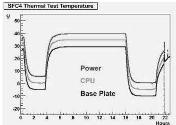
Fig. 5. Temperature variation of SFC in thermal test.
