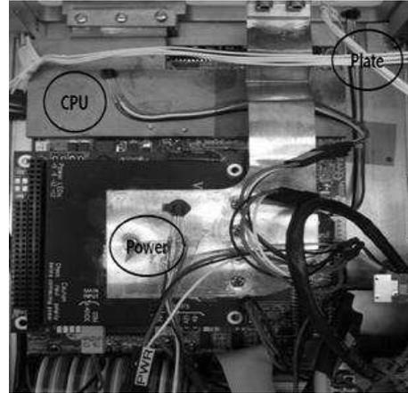
Fig. 3. Science Flight Computer (SFC). Notice three temperature sensors attached on plate, CPU and power module.
