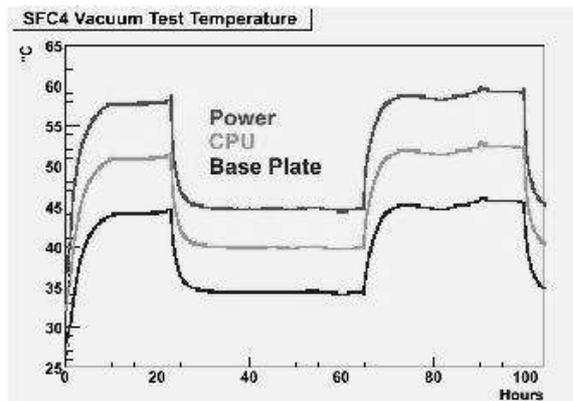
Fig. 4. Temperature variation of SFC in vacuum test.
