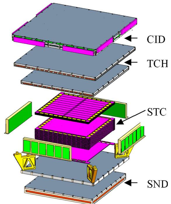
Fig. 3: Expanded view of one HEPCaT module
