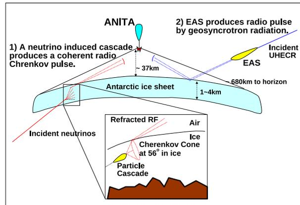
Fig. 1. ANITA Concept for Neutrino and EAS Detection
