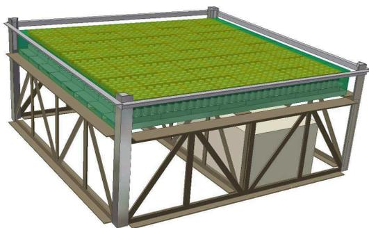
Fig. 3: CREST detector schematic showing the frame with communications box below, the  $32 \times 32$   $\text{BaF}_2$  crystal array, and plastic scintillator veto counters surrounding the crystal volume.
