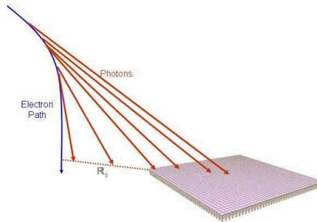
Fig. 2: CREST measurement technique concept. CREST will detect the synchrotron radiation emitted by cosmic-ray electrons as they bend in the Earth’s magnetic field. See text for details.
