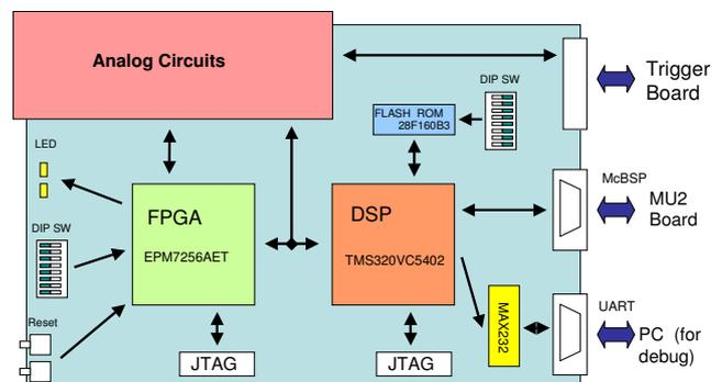
Fig. 3. A block diagram of the BESS-Polar TDC board.
