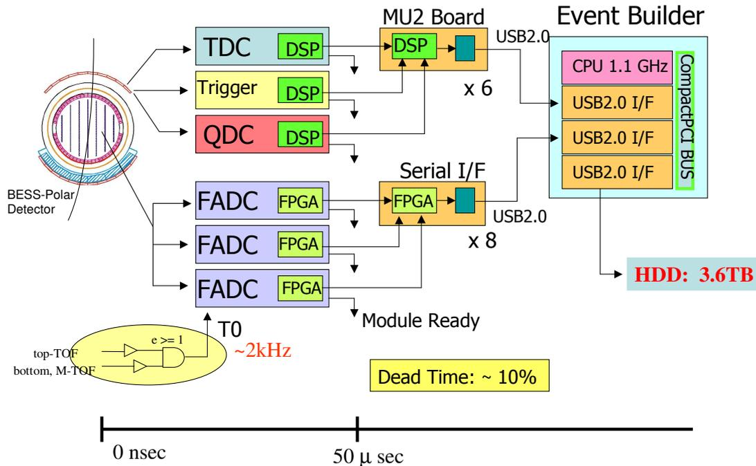
Fig. 1. A block diagram of the BESS-Polar I DAQ system. For the BESS-Polar II, new CPU board with Core Duo 1.66 GHz was used and HDD capacity increased to 16 TBytes. Also, each FADC had the Serial I/F.
