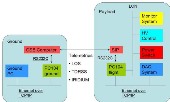
Fig. 4. A block diagram of the BESS-Polar communication flow.
