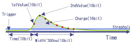
Fig. 2. A schematic view of drift chamber signal and FADC compression value.
