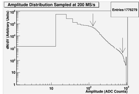
Fig. 5. Amplitude distribution of inclusive amplitude-over-threshold signals measured with the first HAWC WCD prototype with our DAQ system at a sampling rate of 200 MS/s. Each ADC count is equal to 2mV.
