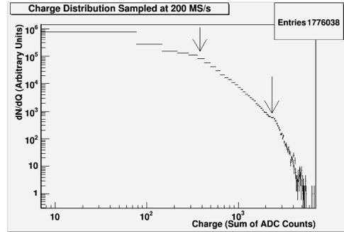
Fig. 4. Charge distribution of inclusive amplitude-over-threshold signals measured with the first HAWC WCD prototype with our DAQ system at a sampling rate of 200 MS/s.
