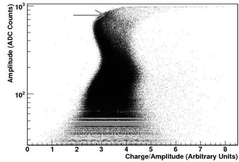
Fig. 8. Amplitude vs charge/amplitude of inclusive amplitude-over-threshold signals measured with the first HAWC WCD prototype at a sampling rate of 200 MS/s. The arrow shows the position corresponding to the right-side arrows shown in Fig. 4 and Fig. 5.
