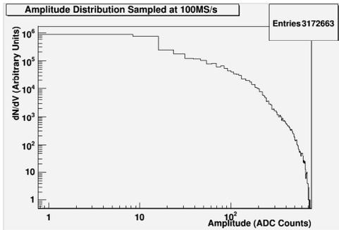
Fig. 7. Amplitude distribution of inclusive amplitude-over-threshold signals measured with the first HAWC WCD prototype with our DAQ system at a sampling rate of 100 MS/s. Each ADC count is equal to 2mV.
