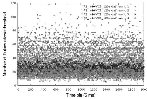
Fig. 2. Rates measured with the first HAWC WCD prototype as taken with our DAQ system. The four thresholds were set at 18, 28, 68 and 108 mV above the baseline. The Y axis shows the number of pulses above each threshold for the 5ms intervals shown on the X axis.
