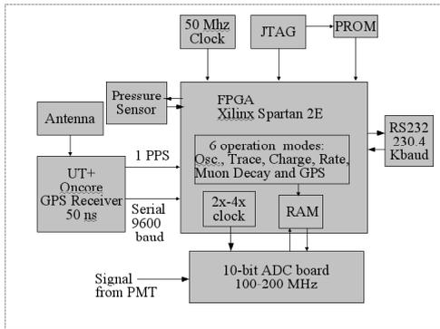
Fig. 1. Schematic diagram of the DAQ hardware.
