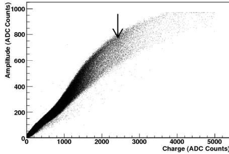
Fig. 6. Amplitude vs charge of inclusive amplitude-over-threshold signals measured with the first HAWC WCD prototype at a sampling rate of 200 MS/s. The arrow shows the position corresponding to the right-side arrows shown in Fig. 4 and Fig. 5.
