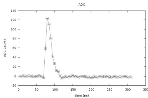
Fig. 3. Typical waveform from the first HAWC WCD prototype as sampled with our system at 200 MS/s. The pulse shape is widened by the shaper of the ADC module. Each ADC count is equal to 2mV.
