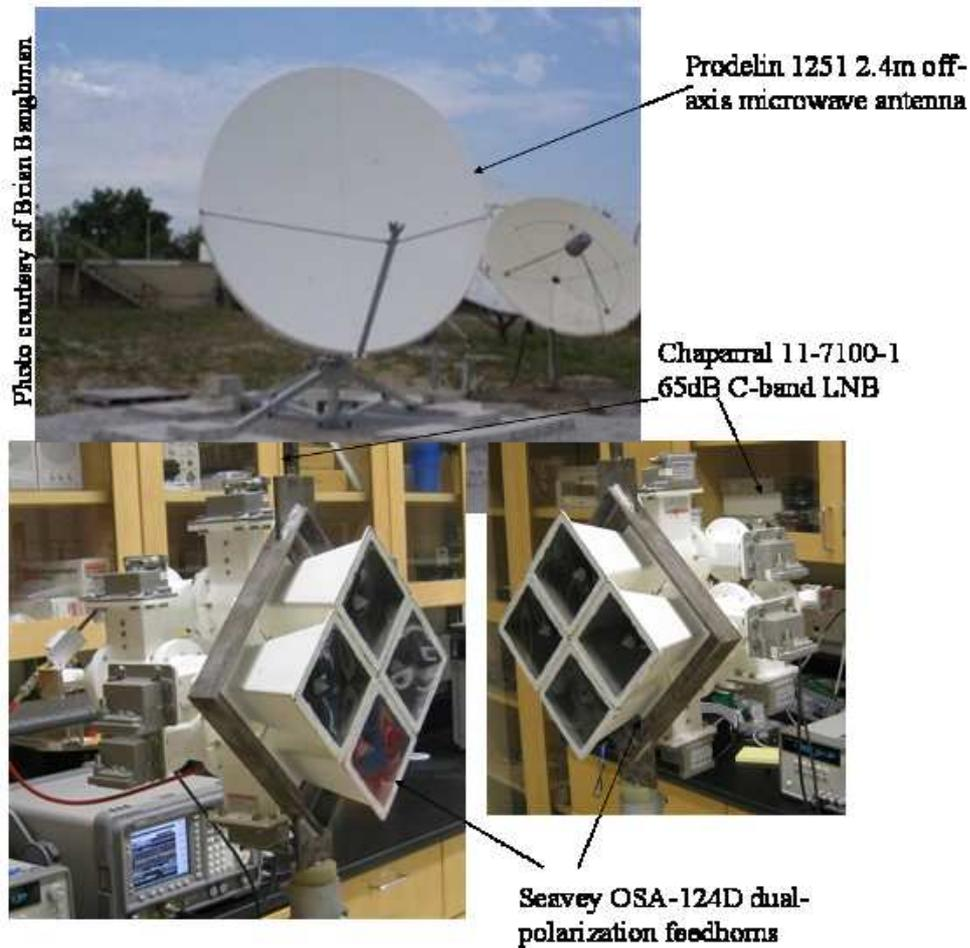
Fig. 1. The prototype feedhorn array at OSU
