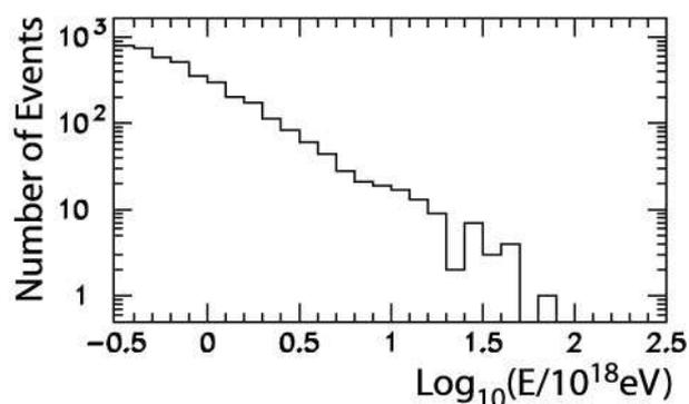
Fig. 7. Distribution of reconstructed  $\log_{10}(E/10^{18}\text{eV})$  for events above  $10^{17.5}$  eV, seen by the TA Middle Drum FD station.
