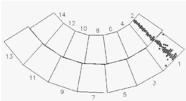
Fig. 3. The diagram of the two-layer layout of the Middle Drum telescopes. The telescopes on the left of the diagram are pointing south. The lower and upper edges of the telescope coverage are at  $3^\circ$  and  $31^\circ$ , respectively. The two right most telescopes are displaying an event from a vertical xenon flasher.
