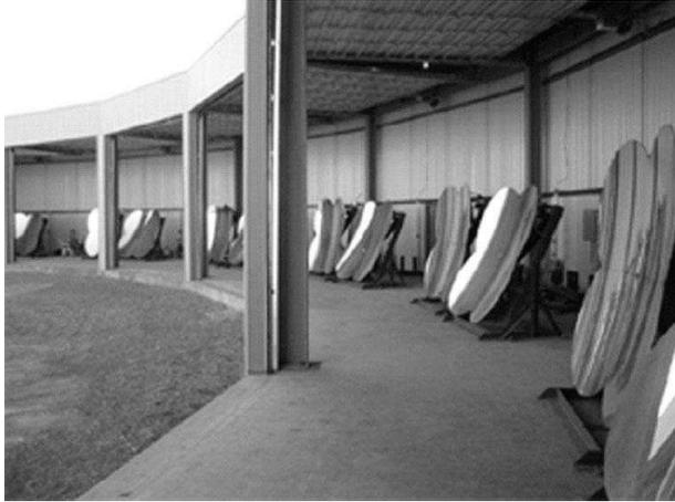
Fig. 2. Photograph of the Middle Drum FD mirror building before PMT cameras were installed. The 14 mirrors are pointed alternately at  $10^\circ$  and  $24^\circ$  to provide overall coverage between  $3^\circ$ – $31^\circ$  in elevation and  $114^\circ$  in azimuth toward the SD array.
