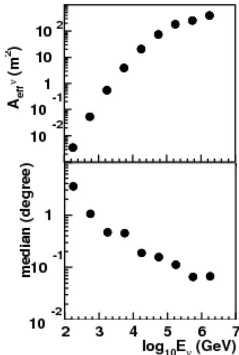
Fig. 1: Neutrino effective areas (top panel) and median of the angle between simulated and reconstructed muon directions (bottom panel) as a function of the neutrino energy for a 127 tower 180m spaced geometry (see text).
