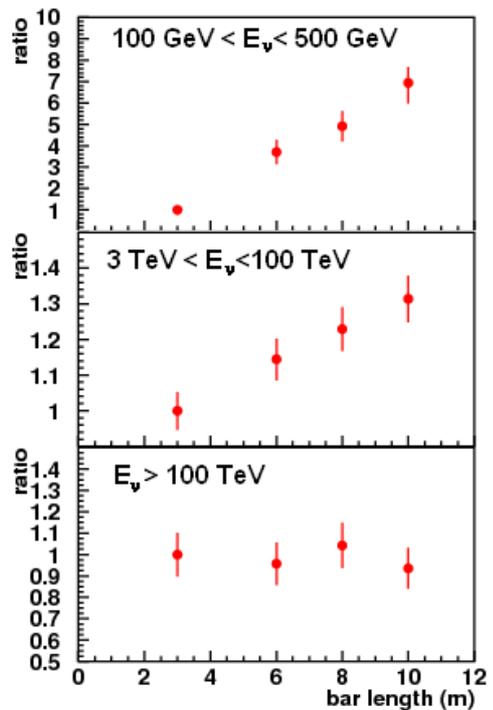
Fig. 4: Ratio of neutrino effective areas with respect to the 3m bar length structure is reported as function of the bar length for different energy ranges. Quality cuts are applied for top and middle panels (see text).
