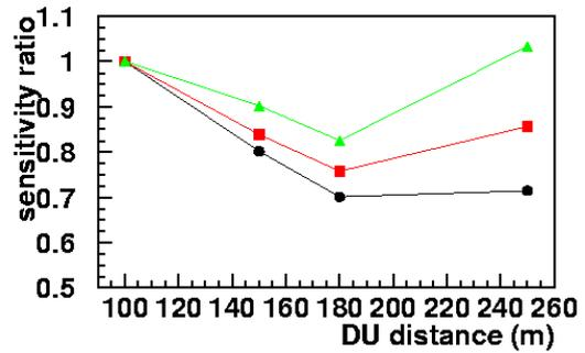
Fig. 3: Ratio of sensitivity to point-like sources with respect to 100m tower distance sensitivity as a function of tower distance for three different spectral indexes. Circles  $\alpha = 1.8$ , squares  $\alpha = 2$ , triangle  $\alpha = 2.2$ .
