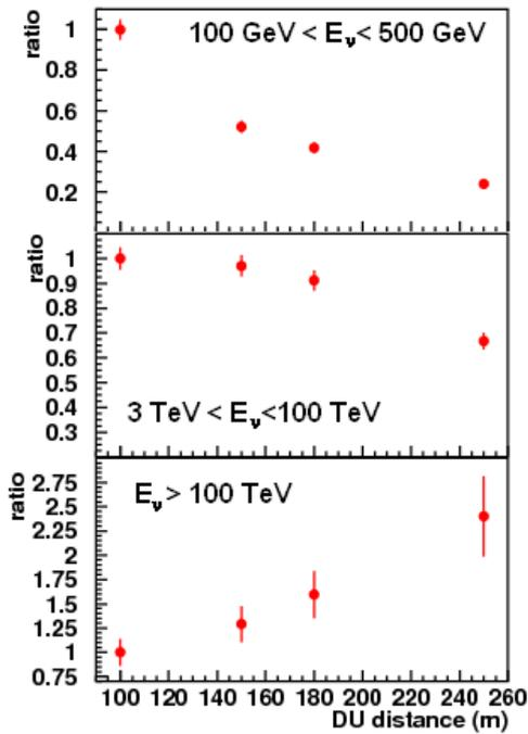
Fig. 2: Ratio of neutrino effective areas with respect to the 100m tower spacing is reported as function of the tower spacing for different energy ranges. Quality cuts are applied for top and middle panels (see text).
