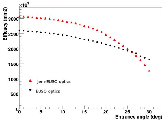
Fig. 3. Effective area of JEM-EUSO (Triangles) compared with EUSO (Dots).
