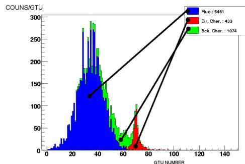
Fig. 2. Profile of the different light components reaching the JEM-EUSO pupil. The event shown has an energy of  $E \sim 10^{20}$  eV and incidence angle  $\theta = 60^\circ$ . The fluorescence component contributes to 78% of the observed light. The peak on the right correspond to the diffusively reflected Cherenkov light. The Gate Time Unit (GTU) is  $2.5 \mu s$ .
