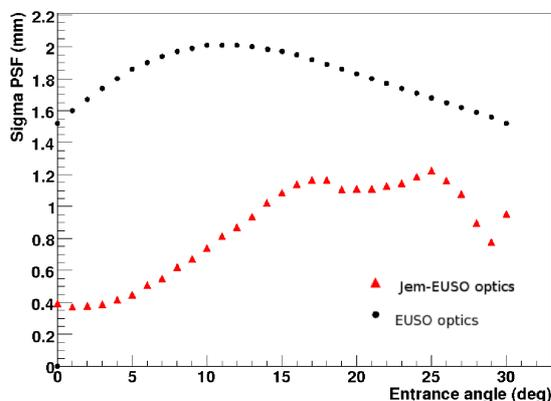
Fig. 4. Sigma of the spot of JEM-EUSO (Triangles) compared with EUSO (Dots).
