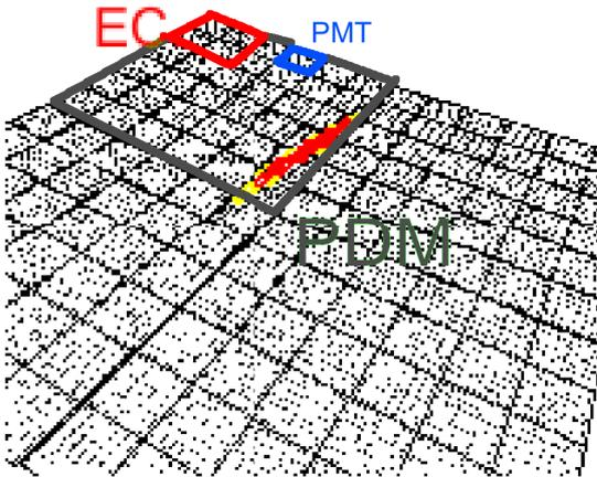
Fig. 5. Integrated track of a  $8 \times 10^{20}$  eV. The detail of the Elementary Cell (EC), of Photo Detector Module (PDM) and of Photomultiplier (PMT) is shown.
