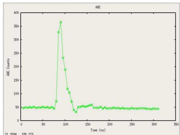
Fig. 6. Signal coming from the detector when a 200 MSPS DAQ system was used in one of the Proto-Hawc detectors.
