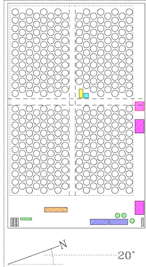
Fig. 3. HAWC at Parque Pico de Orizaba and layout, individual detectors of depth of 4.5 m of water, arranged in a grid of  $22 \times 16$  cylindrical cells of 7.3 m diameter, each one optically isolated from the others.
