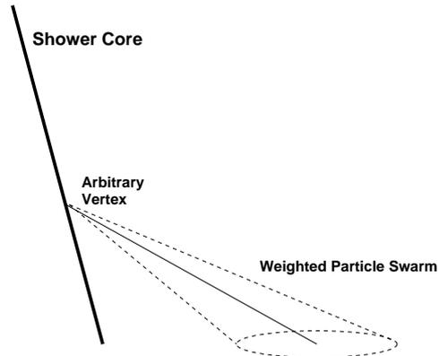
Fig. 1. Geometry for a “Gaussian cone” with an vertex placed at arbitrary position on the shower axis
