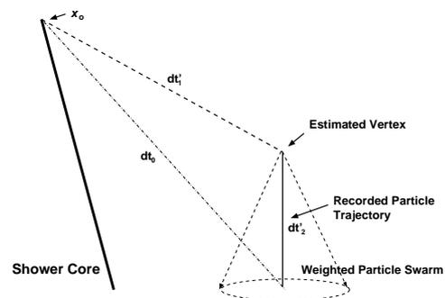
Fig. 3. If  $dt_0 + t_f < dt'_1 + dt'_2$ , where  $t_f$  is the delay between the onset of the EAS and arrival of the weighted particle, the sampled trajectory will always arrive after EAS onset.
