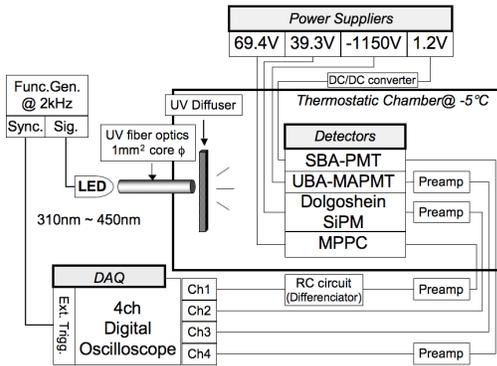
Fig. 4. Schematic diagram of the PDE measurement.
