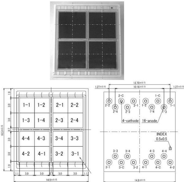
Fig. 1. Top : Photo of 16 ch MPPC array module. Bottom, Left/Right : Blue print of 16ch ( $4 \times 4$ ) of  $3 \times 3 \text{ mm}^2$  MPPC array device (front/back).
