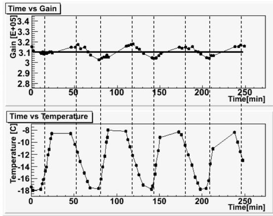
Fig. 8. The top panel shows the gain of a MPPC as a function of time [min] for a cyclic variation of the device temperature [ $^{\circ}\text{C}$ ] (see bottom panel).
