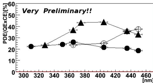
Fig. 5. Preliminary result of PDE measurements. The filled triangles, open circles, and filled circles show the distribution of the Dolgoshein SiPM, the MPPC, and the MAPMT respectively. The PDE is calculated from the ratio of the normalized number of detected photoelectrons in the considered device and in a reference PMT, assuming Poisson distributions. Systematic uncertainties are not shown. Other factors to be considered include the SiPM overvoltage and temperature dependence.
