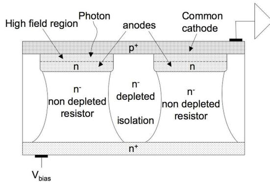
Fig. 3. Concept figure of bulk integrated quench resistor type SiPM (SiMPI).
