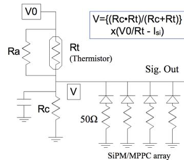
Fig. 6. Temperature compensation circuit with a thermistor (Rt).
