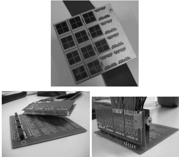
Fig. 9. 256 ch prototype camera with  $4 \times 4$  MPPC array module. The circuit module consists of one mother board and four daughter boards to simplify the further modification.
