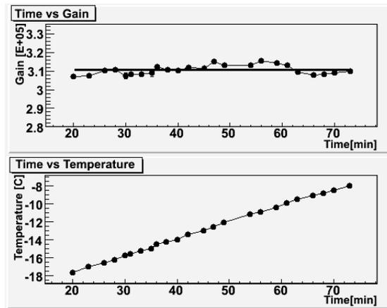
Fig. 7. The top panel shows the gain of a MPPC as a function of time [min] for a gradual increase of the device temperature [ $^{\circ}\text{C}$ ] (see bottom panel).
