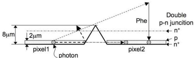
Fig. 2. Schematic view of “prompt” and “slow” optical crosstalk (OC) and the concept of OC suppression.
