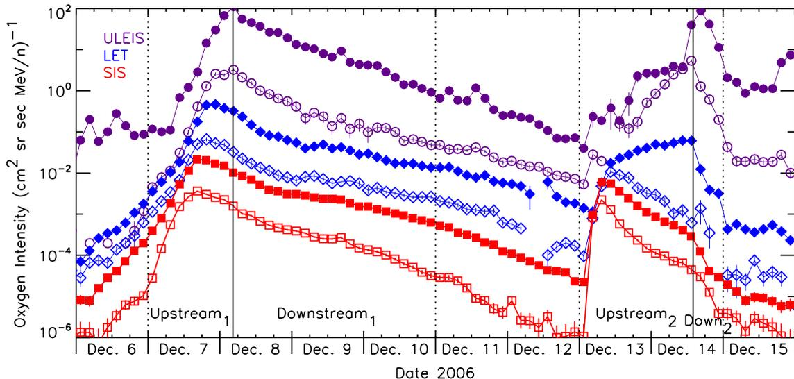
Fig. 1: Three-hour averaged O intensities from ULEIS (circles) at 0.14 (solid) and 1.5 (open) MeV/n, LET (diamonds) at 4.9 (solid) and 12 (open) MeV/n, and SIS (squares) at 18 (solid) and 34 (open) MeV/n. Solid lines mark shock passages and dashed lines mark boundaries of the selected upstream and downstream regions.
