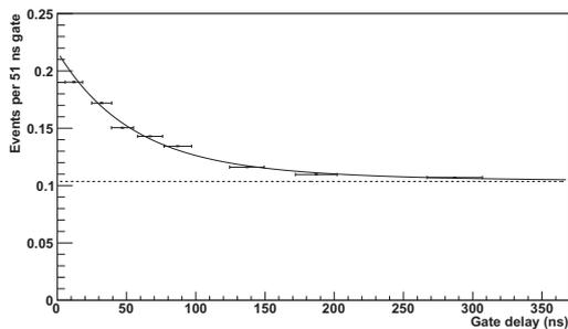
Fig. 2: Number of afterpulses of a G-APD for variable gate delays after an initial breakdown: the afterpulse rate is exponentially decreasing. The dashed line indicates the amount of dark counts. Taken from [2].
