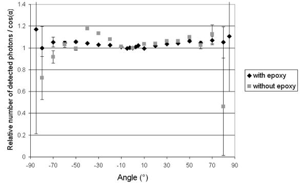
Fig. 4: Relative photon detection efficiency for different incident angles of a pulsed light flash. The G-APD is coated by a protective epoxy layer. Due to refraction, the incident angle at the chip surface is around 40° for an inclination of the light beam of 85°.
