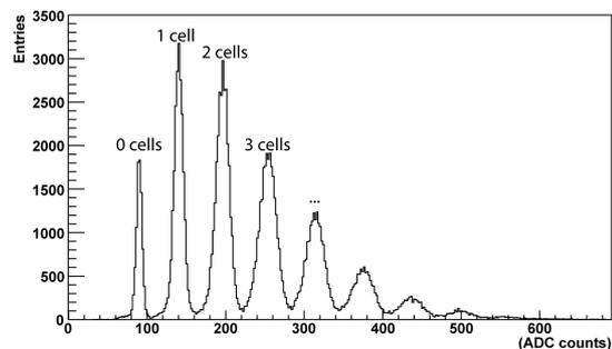
Fig. 1: Pulse spectrum of a weak pulsed LED measured with a G-APD. The peaks correspond to the number of triggered cells  $\bar{N}$  according to equation (3). Taken from [2].
