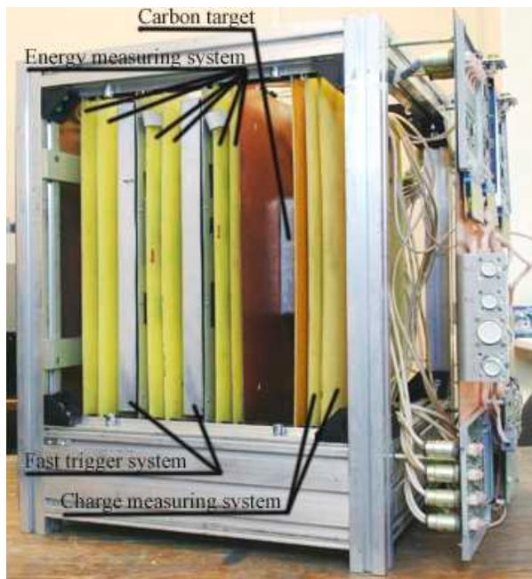
Fig. 1: Side view of the NUCLEON device design.
