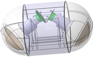
Fig. 2: The "capsule" Optical Module.
