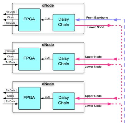
Fig. 3: Scheme of the daisy chain architecture.
