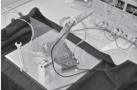
Fig. 3: Setup to measure the angular efficiency of the light concentrators. A pulsed LED is mounted on the metal bar in the foreground. The angle relative to the vertical direction can be read from a transparent angular scale. This lever is mounted on a common base plate with the board holding G-APDs, electronic amplification and light guides. Special holes in the base plate allow measuring selected input orientations (parallel to a G-APD edge or to the diagonal).
