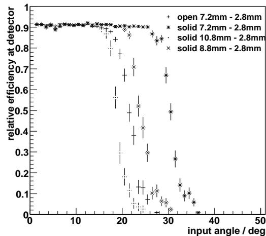
Fig. 2: Comparison of an open and solid CPC ( $n = 1.5$ ) with an area concentration factor  $C = 6.6$ , as well as solid CPCs with  $C = 14.9$  and  $C = 9.9$ . 5% reflection losses were assumed for both types. Error bars are purely statistical and indicate variations caused by different input points on the entrance area and different directions  $\phi$ .
