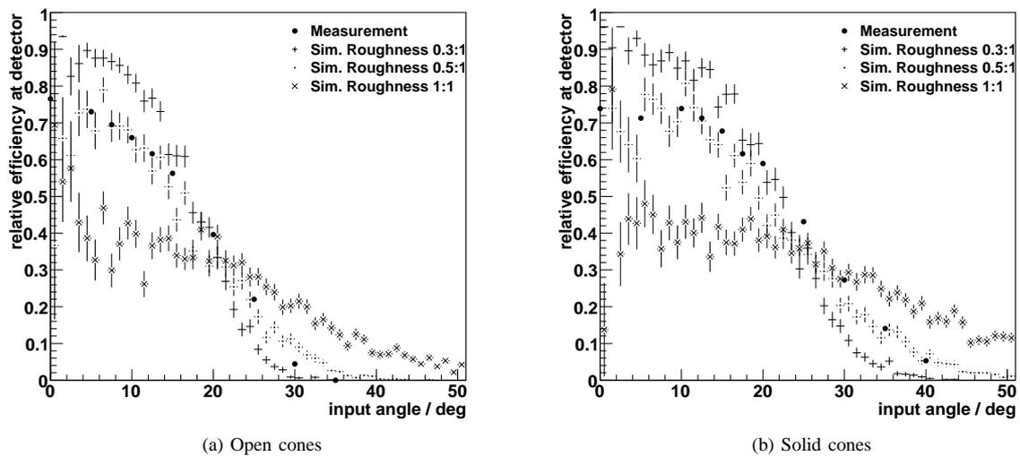
Fig. 5: Angular acceptance curves for different surface roughness (0.3:1, 0.5:1, 1:1) for pyramidic cones compared to measurements (rescaled).
