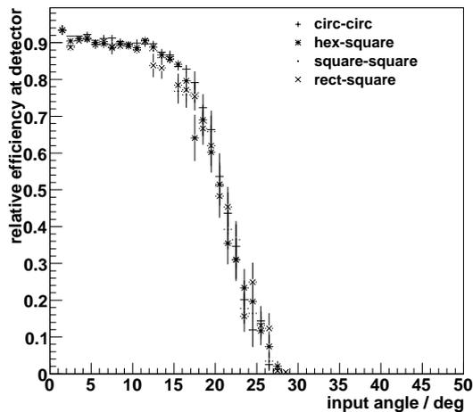
Fig. 1: Comparison of parabolic concentrators with different input and output shapes, but the same concentration factor of 6.6. The first phrase in the legend denotes the shape of the input area, the second phrase the output area (circ=circular, hex=hexagonal, square=quadratic and rect=rectangular shape).
