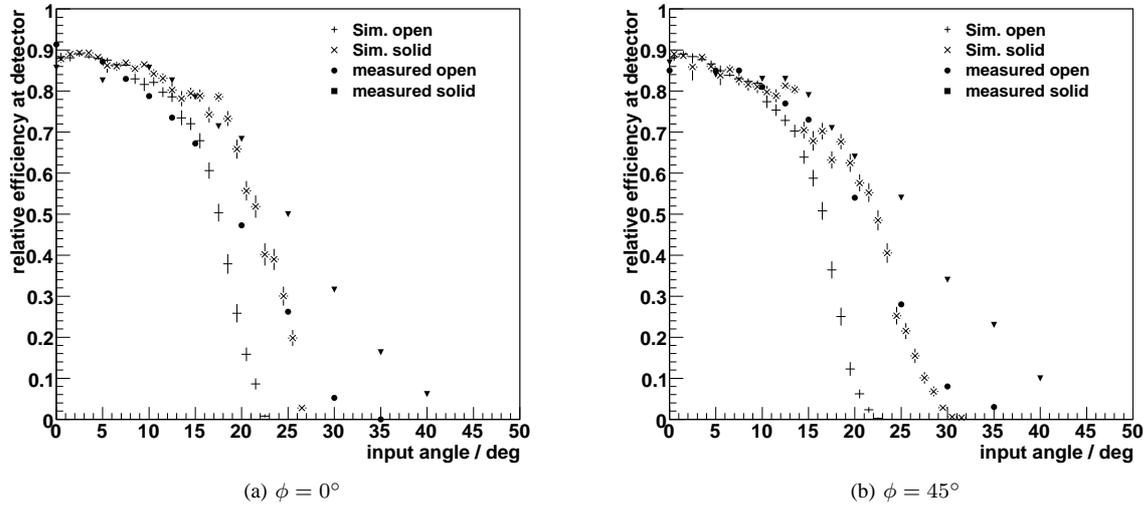
Fig. 4: Comparison between simulated angular acceptance curves and measurements (rescaled) for pyramidic cones. Two input directions ( $\phi = 0^\circ$  and  $\phi = 45^\circ$ ) were measured for each prototype.
