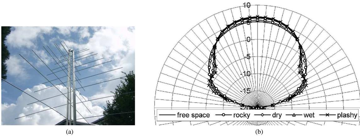
Fig. 3: (a) Logarithmic Periodic Dipole Antennas (LPDA), (b) its E-plane directional diagram as in Fig. 2b.
