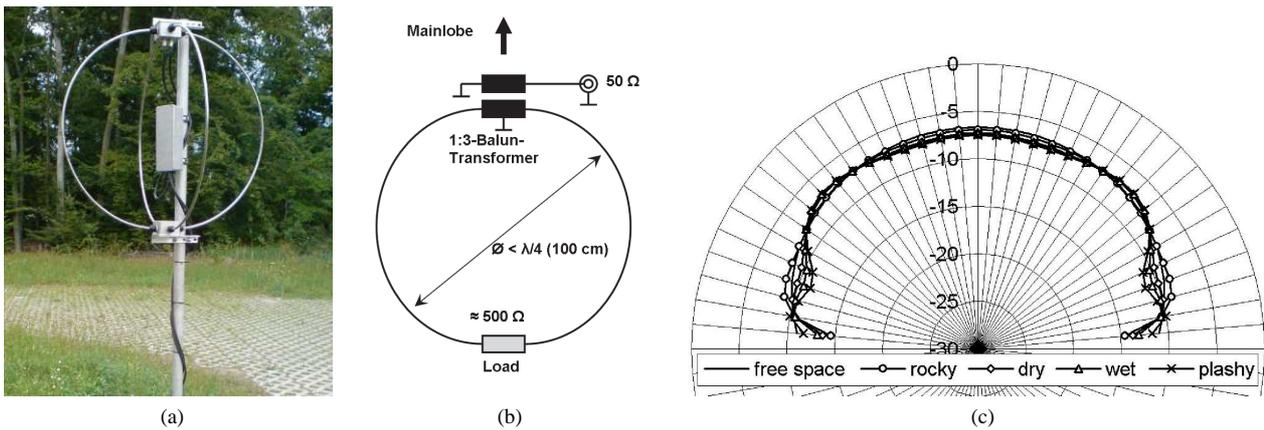
Fig. 4: (a) Short Aperiodic Loaded Loop Antenna (SALLA), (b) its principle, (c) and its E-plane directional diagram.
