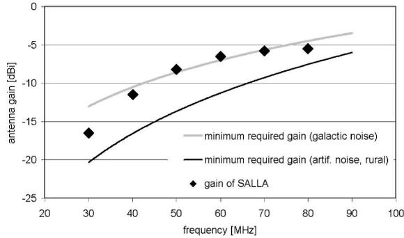
Fig. 5: Minimum required antenna gain without significant lowering the signal-to-noise ratio for external galactic noise (grey) and for man-made noise (black: rural environment) including a characteristic noise of the preamplifier of  $2\text{ dB}$ . Frequency dependent galactic noise temperatures are derived from [3].
