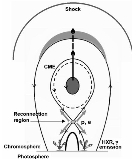
Fig. 5. Schematic of a solar flare, including the reconnection region where energy is released and particles accelerated, the chromospheric foot-points where x-rays and  $\gamma$ -rays are produced, a CME and CME-driven shock. ENAs are produced wherever there are accelerated particles, with a yield proportional to the energetic-particle and ambient densities (adapted from a RHESSI Science Nugget [18]).
