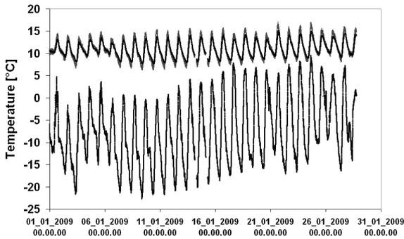
Fig. 3: Monitoring of the external temperature (lower plot), of the inner temperature close to the ARGO-YBJ carpet center (upper plot, background), and of the temperature on the output gas line of a chamber (upper plot, foreground) at the YangBaJing site from January 1 till January 28, 2009.
