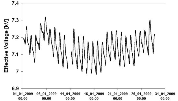
Fig. 5: Time trend of the effective voltage applied to the RPC detectors if reference temperature 12 °C and reference barometric pressure 600 mbar are chosen. The short maintenance break in the detector operation mentioned in the caption of Fig. 4 is visible.
