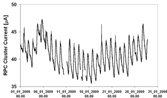
Fig. 4: Time trend of the ARGO-YBJ RPC cluster current over 29 days in January, 2009. Each point represents the mean value over one minute. An interruption in the monitoring due to maintenance operations on the detector is visible.
