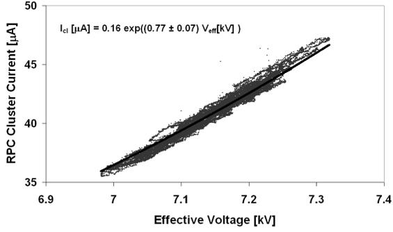
Fig. 6: Scatter plot of the RPC cluster current versus the RPC effective voltage. A very good linear correlation between the effective voltage and the logarithm of the current is established, with linear correlation coefficient equal to 0.99.
