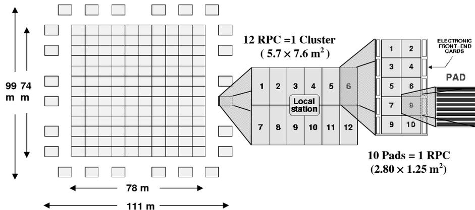
Fig. 1: Scheme of the ARGO-YBJ detector layout, with the details of its structure.
