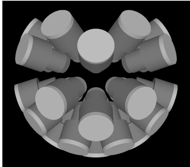
Fig. 2. The GEANT4 model of the KM3NeT Multi-PMT optical with 31 PMTs.
