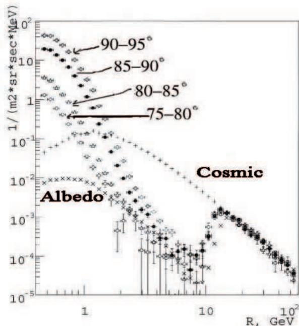
Fig. 2: Proton spectra for different pitch-angles for  $B < 0.216G$ ,  $L < 1.5$ .
