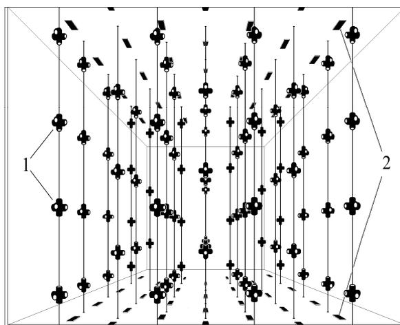
Fig. 2: Detecting system of CWD NEVOD. 1 – quasispherical modules, 2 – scintillation telescopes.
