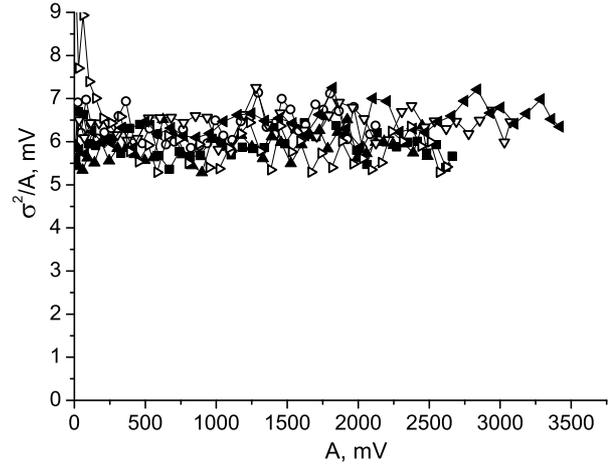
Fig. 4: Behavior of the conversion factors of six spectrometric circuits as a function of output amplitude.
