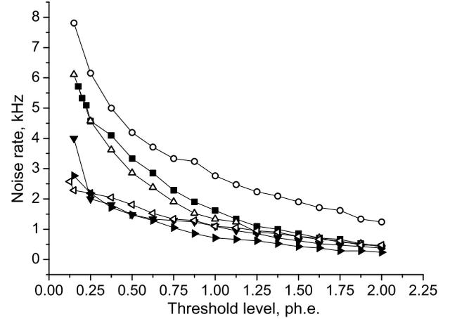
Fig. 5: Dark noise rate of six FEU-200 PMT for different thresholds of the discriminator.
