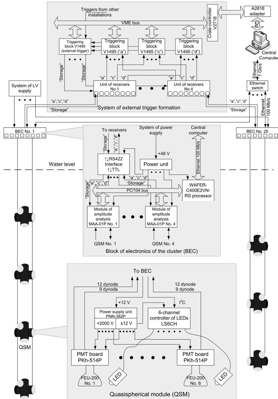
Fig. 3: Scheme of the new measuring system.
