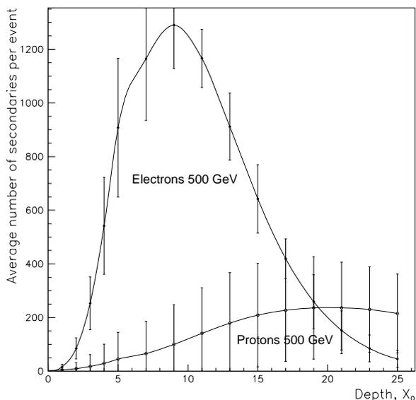
Fig. 2: Comparison of average electron and proton cascades in the calorimeter
