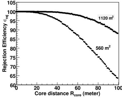
Fig. 3: Rejection efficiency as a function of core distance of the showers from center of the muon detector. The upper curve is for the expanded muon detector and the lower curve is the for the present muon detector
