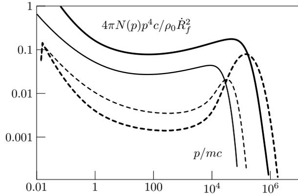
Fig. 3: Spectra of accelerated protons (thick lines) and electrons (multiplied on 5000, thin lines) at  $t = 1050$  yr. Spectra at the forward shock (solid lines) and at the backward shock (dashed lines) are shown.
