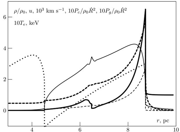
Fig. 2: Radial dependencies of the gas density (thick solid line), the gas velocity (dotted line), CR pressure (thick dashed line), the gas pressure (dashed line) and the electron temperature (thin solid line) at  $t = 1050$  yr. At this moment of time the forward shock velocity is  $3540 \text{ km s}^{-1}$ , its radius is  $8.7 \text{ pc}$ , the magnetic field strength downstream of the forward shock is  $146 \mu\text{G}$ .
