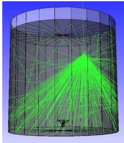
Fig. 2. Simulated 100MeV gamma-ray showering in a HAWC tank. The depth of the water must be sufficient that secondary shower particles never pass close to the PMTs producing large pulses that could be misidentified as muons.
