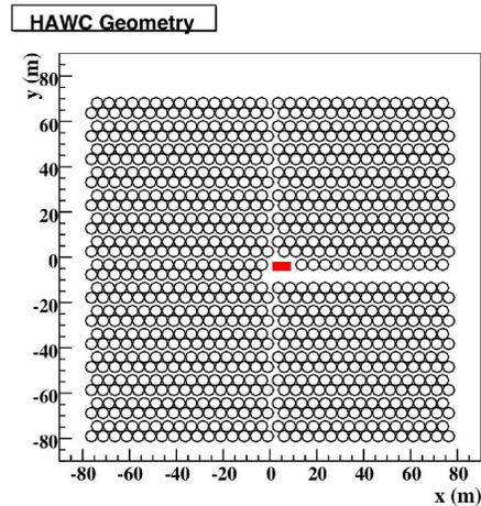
Fig. 1. Proposed layout of the HAWC detector. A dense array of 900 5m diameter water tanks will be deployed over an area of 25000m<sup>2</sup>. The counting house will be situated in the middle of the array to minimize the length of the cables.
