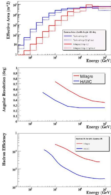
Fig. 5. Comparison of Milagro (red) and HAWC (blue) sensitivity. HAWC will see large improvements in effective area, angular resolution and gamma/hadron separation compared to Milagro.
