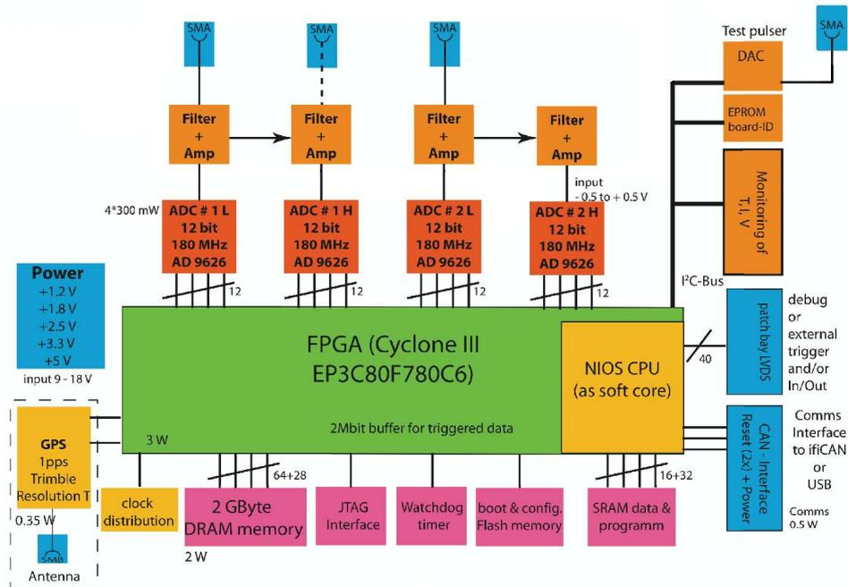
Fig. 3: Block diagram of new electronics design
