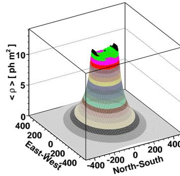
Fig. 1. The mean density of Cherenkov light for all produced photons in  $\gamma$  cascades - primary energy of 100 GeV
