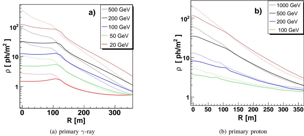
Fig. 2. Comparison between the average lateral density distributions obtained at observations levels of 2.2 km (solid lines) and 4.0 km (dotted lines)
