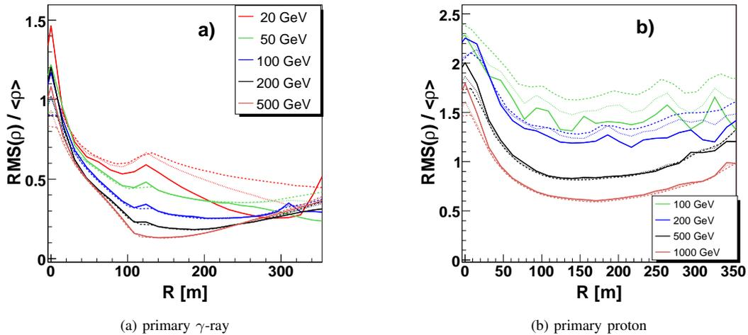
Fig. 4. The relative dispersions of the Cherenkov light density obtained for different detector sizes: 240 (solid lines), 480 (dotted lines) and 960  $m^2$  (dashed lines) at the observation height of 2.2 km
