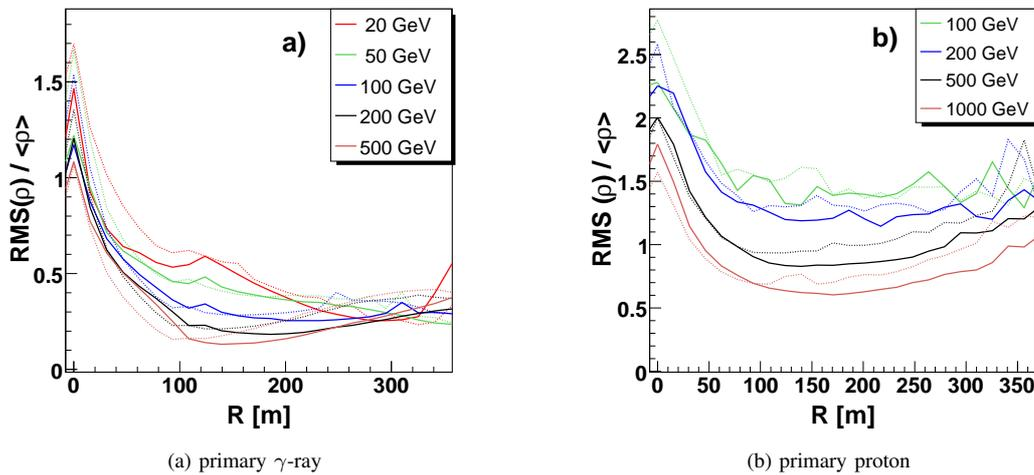
Fig. 3. The expected relative dispersions of the Cherenkov light density on the ground for detector size of  $240m^2$ ; solid and dotted lines correspond to the observation altitude of 2.2 km and 4 km, respectively.
