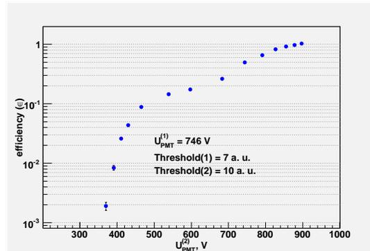
Fig. 2. Rejection efficiency dependence on a PMT HV tension for down-stream plane
