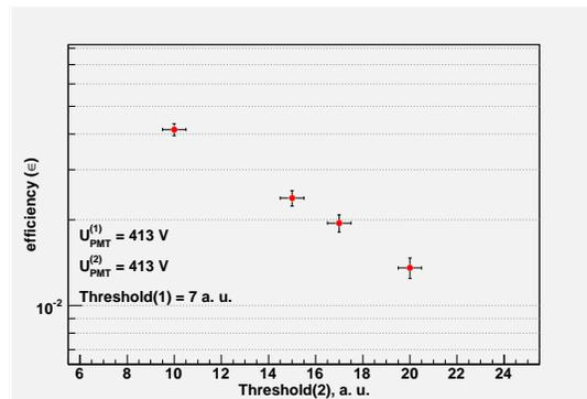
Fig. 3. Rejection efficiency dependence on a threshold of down-stream plane
