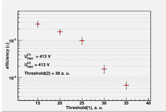
Fig. 4. Rejection efficiency dependence on a threshold of up-stream plane
