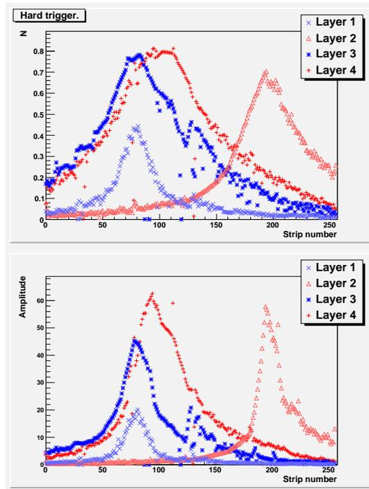
Fig. 6. The normalized integral distributions of hit strips with the hard trigger conditions
