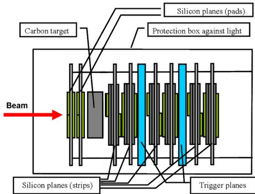
Fig. 1. The NUCLEON prototype on the beam in the CERN SPS
