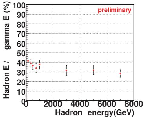
Fig. 7: For the hadron incident events, the number of detection particle become less compared with the same energy of electron event because of the shower leakage. The longitudinal axis shows the ratio of  $E$  of neutron and  $E$  of gamma-ray event.
