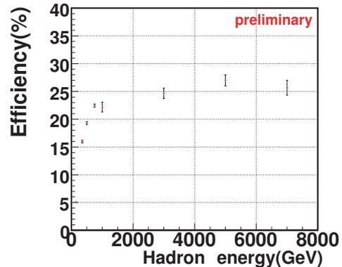
Fig. 5: Detection efficiency of neutron incident events. The threshold of detection is defined that any successive three layers record more than 150 MeV. For high energy, the detection efficiency is around 25%.
