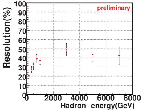
Fig. 6: Energy resolution for neutron events. The energy resolution is about 40 % in high energy.
