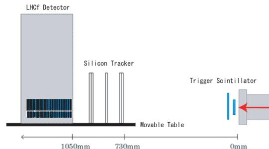
Fig. 3: Setup of the SPS experiment. Beam enters from right along the arrow. Two plastic scintillators were used to trigger beam particles. The silicon tracker, ADAMO [4], was placed in front of the LHCf detector. The two structures shown in the detector are the calorimeters. The detector and ADAMO were placed on a movable stage.
