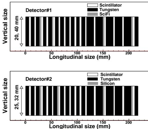
Fig. 1: Longitudinal structure of detector 1 (top) and detector 2 (bottom); black, white, gray boxes indicate the layers of tungsten, plastic scintillator, position sensors (SciFi and Silicon), respectively.
