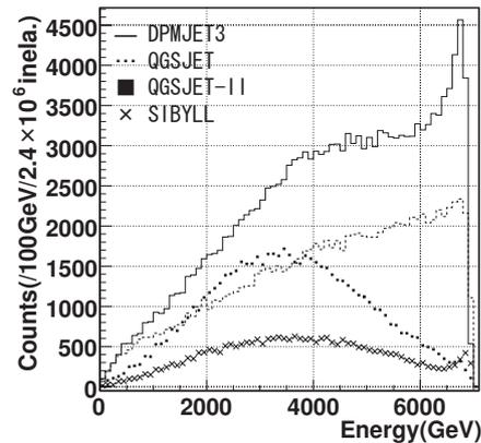
Fig. 2: The energy distribution of neutrons incident on the 20 mm $\times$ 20 mm calorimeter for various models. The calorimeter is positioned at the center of the neutral particle flux.
