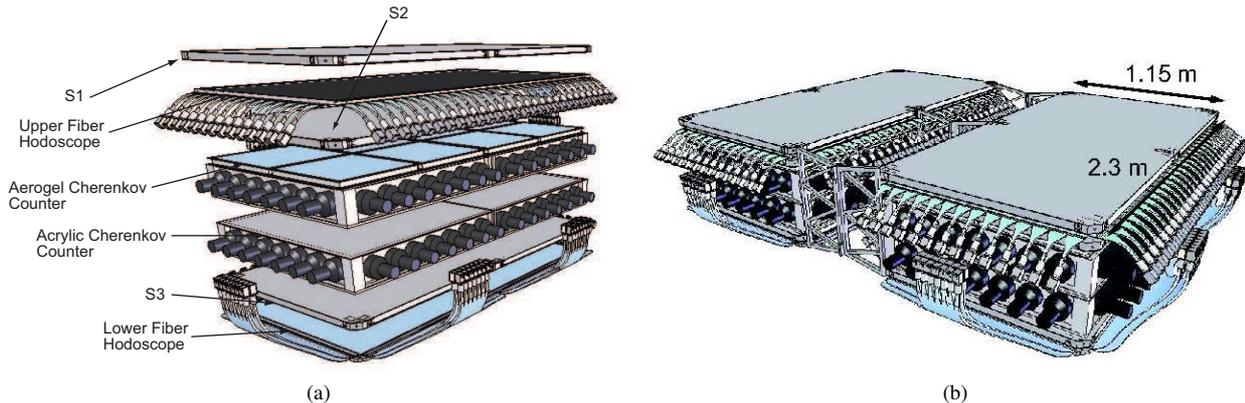
Fig. 1: (a) Exploded view of Super-TIGER instrument. (b) Full Super-TIGER concept (combining 2 modules as shown in (a) together).
