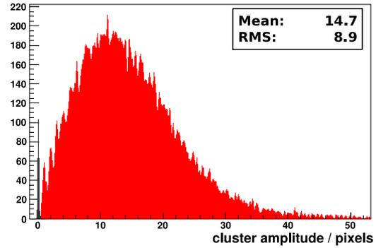
Fig. 5. Stacked signal distribution of an SiPM array exposed to minimally ionizing particles.
