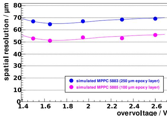
Fig. 9. Expected spatial resolution as a function of the overvoltage for a Hamamatsu MPPC 5883 and for a planned device with a reduced epoxy layer thickness.
