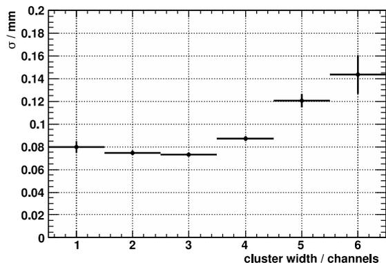
Fig. 8. Spatial resolution as a function of the cluster width.
