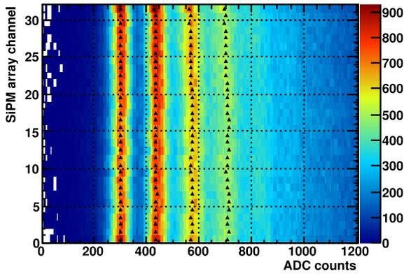
Fig. 4. LED spectra of a 32 channel Hamamatsu MPPC 5883. The center of gravity of the first photoelectron peaks is marked with black triangles.
