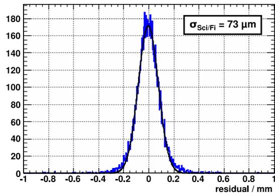
Fig. 7. Spatial resolution of the tested tracker module at 99% efficiency.
