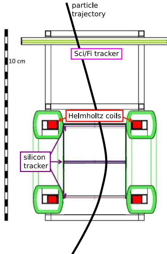
Fig. 1. Drawing of the PEBS-2 spectrometer.
