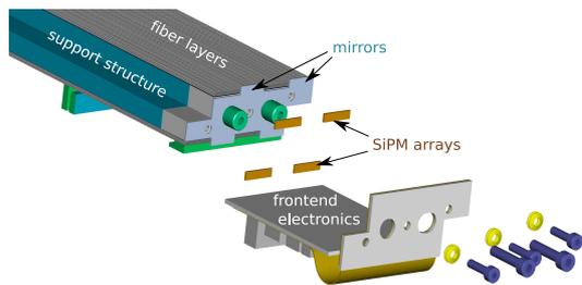
Fig. 2. Exploded drawing of a Sci/Fi tracker module.
