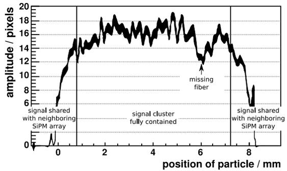
Fig. 6. Light yield along an SiPM array.
