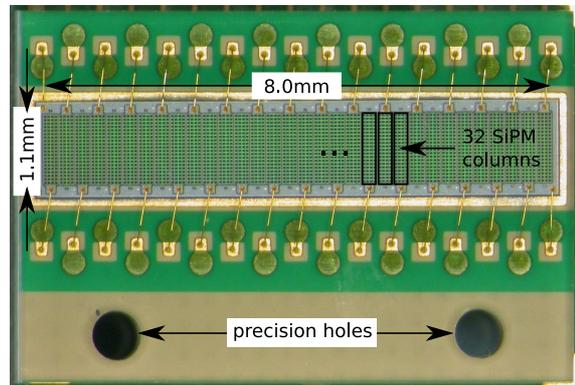
Fig. 3. Microscope picture of a 32 channel Hamamatsu MPPC 5883.
