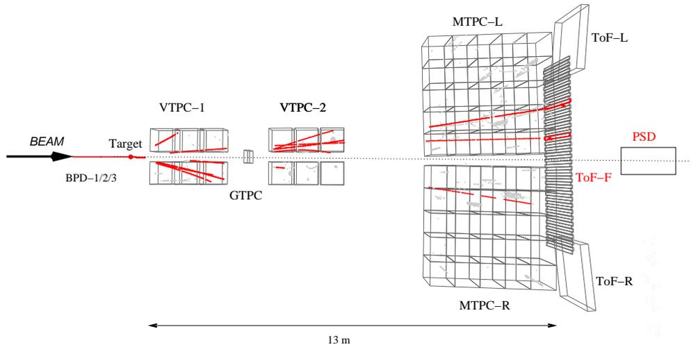
Fig. 2. A typical event recorded during the pilot run for a proton beam (31 GeV/c) on a thin carbon target. The NA61/SHINE detector layout is sketched with the exception of the vertex magnets surrounding the vertex TPCs. Two of the particles have left a signal in the forward ToF detector.
