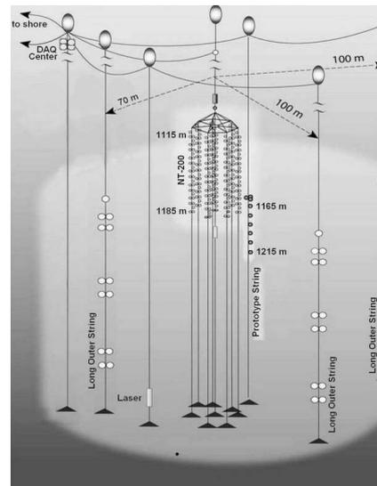
Fig. 1: The Lake Baikal neutrino telescope: the compact NT200 (center), 3 long outer strings and the new technology km<sup>3</sup>-prototype string deployed in 2008.
