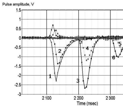
Fig. 4: Example of a LED flasher event detected with all FADC channels
