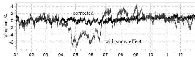
Fig. 7: Distorted by the snow effect and corrected data of the Jungfrauoch station (3nm64) during January - December 2008. The based stations are Jungfrauoch-18IGY (black curve) and Rome (grey curve).
