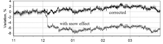
Fig. 2: Distorted by the snow effect and corrected data of Magadan station during November 2008 - April 2009. Black curve for Gaussian smoothing, grey curve - polynomial smoothing. The based station - Moscow.
