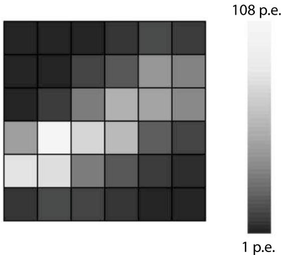
Fig. 3: Simulated air shower induced by a 10 TeV proton (177 m impact parameter,  $1.5^\circ$  incident angle), as seen by the G-APD prototype module. The units of the grayscale axis are photoelectrons (p.e.); one square corresponds to one of the 36 pixels.
