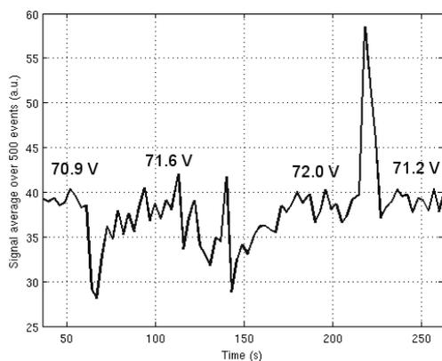
Fig. 5: Demonstration of the functionality of the HV feedback system for one pixel. Under changing light conditions, the G-APD bias voltage was readjusted on-line as indicated (see also text).
