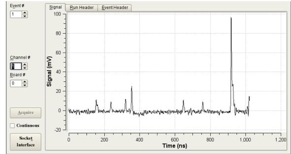
Fig. 4: Online raw data display of the readout system. For one pixel and event, the full DRS2 pipeline of 1024 samples can be seen, containing the signal of a LED pulser and several dark current events.
