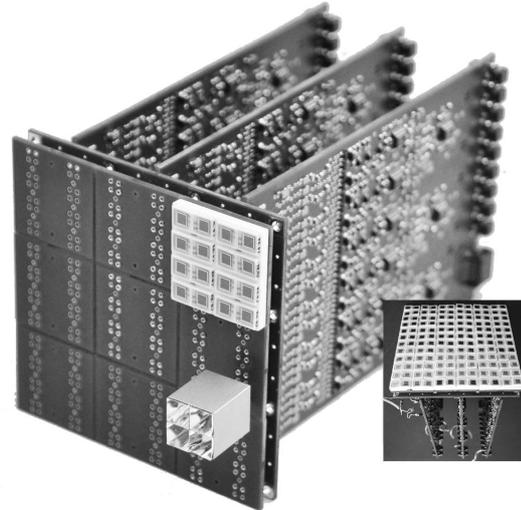
Fig. 2: Photograph of the prototype module with four pixels (16 G-APDs) assembled; for better visibility one block of four Winston Cones is mounted separately. Three amplifier boards are attached directly to the G-APD plane. The small photograph shows the fully assembled G-APD plane without Winston Cones. The active area is  $8.6 \times 8.6 \text{ cm}^2$ .
