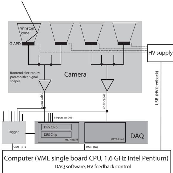
Fig. 1: Schematic overview of the G-APD camera layout (upper part) and the DAQ system (lower part, used in this form for the prototype module). A feedback system is used to regulate the bias voltage of the G-APDs in case of changing observational conditions. The camera will be mounted inside a water-tight box, while the DAQ and trigger components will be located in a counting room.
