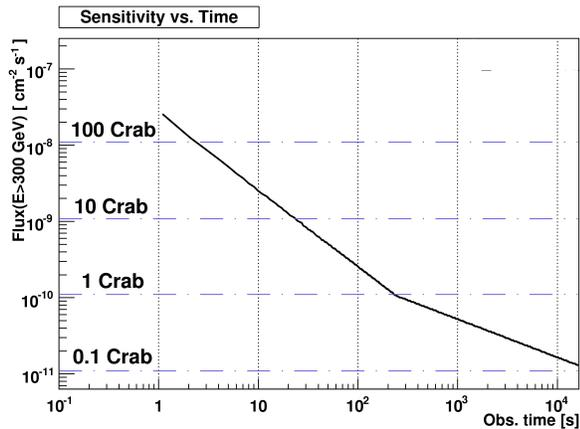
Fig. 1: MAGIC sensitivity corresponding to a  $5\sigma$  detection [15] as a function of exposure time.
