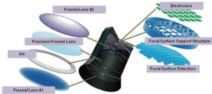
Fig. 1. Schematic view of the JEM-EUSO telescope.
