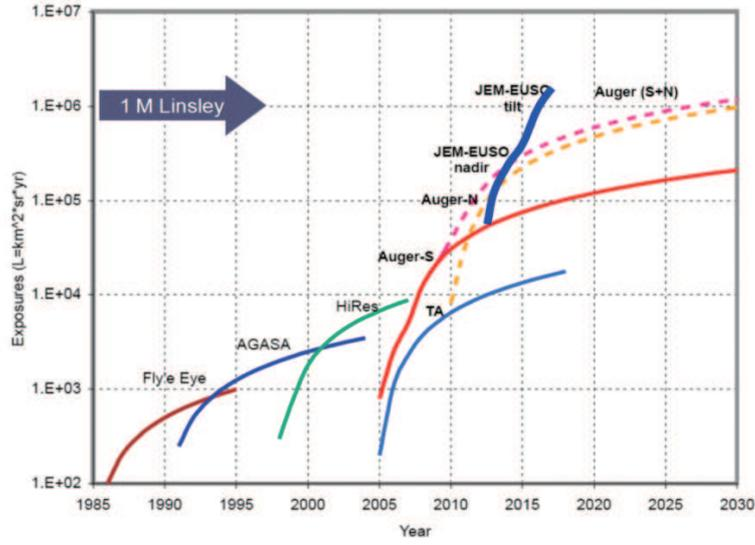
Fig. 3. Expected cumulative exposure, in Linsley units, of JEM-EUSO. For comparison, the evolution of exposures of other retired and running EECR observatories are shown (1 Linsley =  $1 \text{ km}^2 \cdot \text{sr} \cdot \text{year}$ ).
