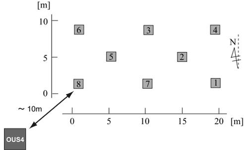
Fig. 1: Detector arrangement of the OUS1 array and the OUS4 array (top view). Numbered squares represent scintillation counters.
