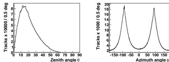
Fig. 3. Reconstructed angular distributions of muons measured with the calibration setup in the surface laboratory. The results are preliminary since reconstructed hit positions were not calibrated yet.
