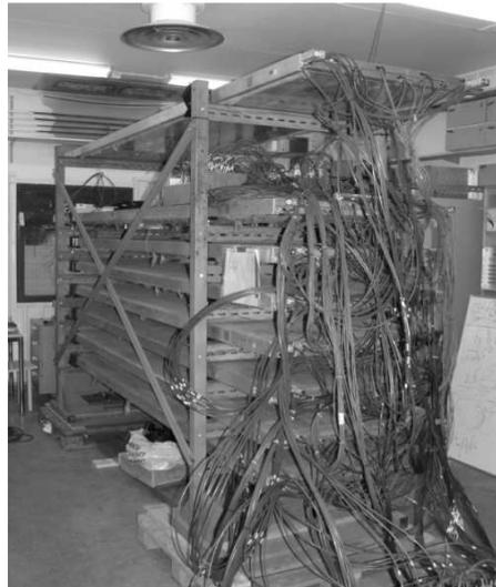
Fig. 2. A calibration setup constructed of eight detector planks in the surface laboratory in Pyhäsalmi.
