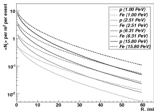
Fig. 5. Average lateral density distributions of high-energy muons of vertical proton and iron showers at different primary energies simulated with CORSIKA-QGSJET01. The threshold energy of muons was 50 GeV which corresponds roughly to the average energy loss of muons in rock.
