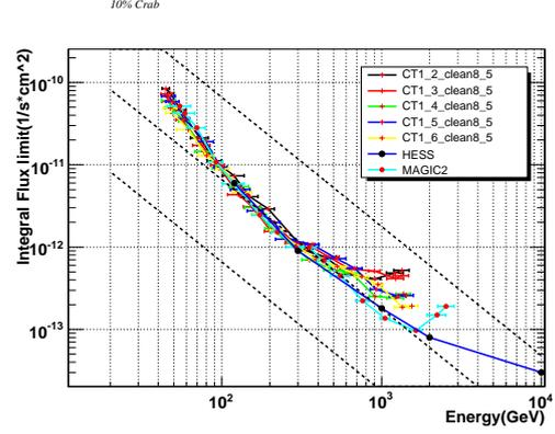
Fig. 8: This plot shows the sensitivities of the two telescopes with different distance. The bright blue line shows MagicII sensitivity and the blue line shows HESS sensitivities.
