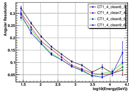
Fig. 5: The angular resolution for different image cleaning parameters. The distance between the two telescopes is 100m.
