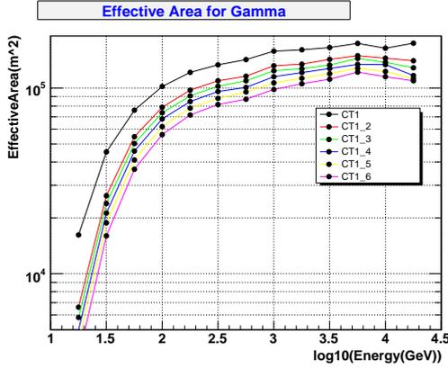
Fig. 1: The effective area for gamma with different distances between the two telescopes of 60m (CT1\_2), 80m (CT1\_3), 100m (CT1\_4), 120m (CT1\_5), 140m (CT1\_6). CT1 indicates the effective area of one telescope.
