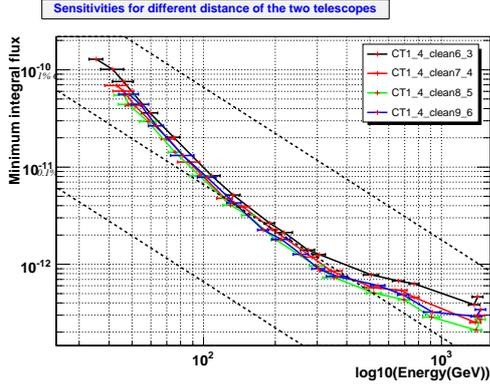
Fig. 6: The sensitivities of the two telescopes with distance 100m for different image cleaning parameters. From this plot the image cleaning parameter 8phe for core pixels and 5 for boundary pixels should be best.
