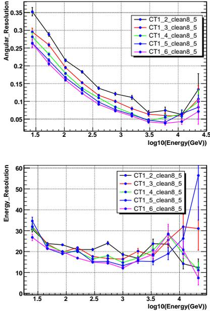
Fig. 7: The upper plot shows angular resolution and the bottom plot shows energy resolution. The angular and energy resolution become better when the distance of the two telescopes becomes longer.
