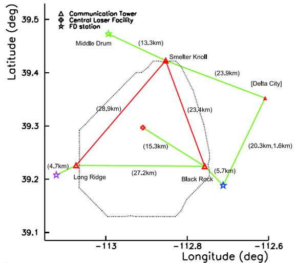
Fig. 1. Area of completed 507 SD array surrounded by 3 FD stations(\*). The  $\Delta$  represents communication tower where the trigger judgment electronics for sub-array are installed. Lines drawn to connect each tower and facilities represents the links between antennas.
