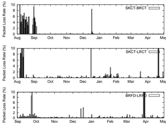
Fig. 5. Long term stability of the network from Aug.2008. Top two panels shows daily packet loss rate at the line of SK to BR tower and SK to LR tower used for SD data acquisition. Bottom panel shows the one at the line of BR FD station to LR FD station.
