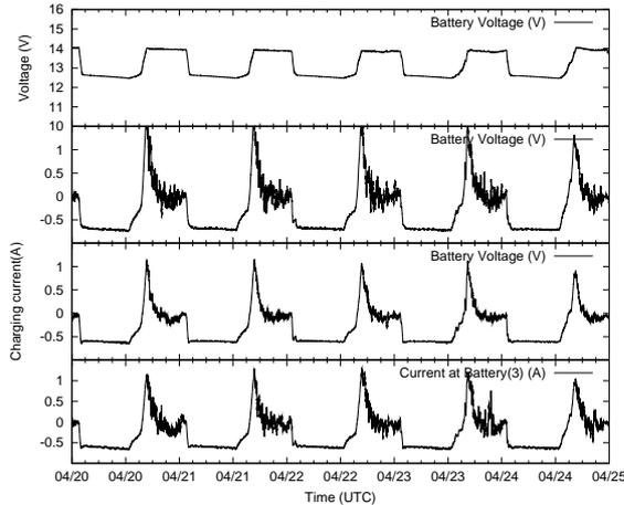
Fig. 4. The example of tower monitor data. Variation of 10 min average of battery voltage and current at battery terminals are plotted along the UTC. It is seen that batteries are charged up to full charge in daytime and discharging in night time.
