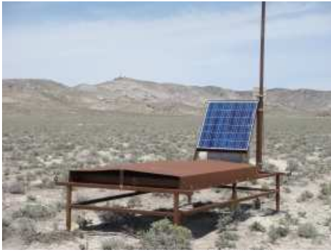
Fig. 2. A picture of deployed SD. Electronics box and scintillator are on the iron frame. Electronics exists under the solar panel and scintillator box exists under the roof visible at the picture. Each SD are deployed in 1.2km of separation.
